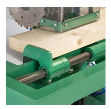
Further, T-KAPP cuts as large as 250x160 mm, so the operator can easily make large cuts for major structures.
